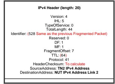
Fragmented IPv4/IPv6/UDP Packet (Last Fragment) (length: 44 bytes)
