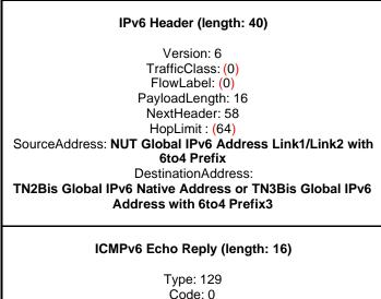
Code: 0 Checksum: To calculate Identifier: (514 Same as the ICMPv6 Echo Request) SequenceNumber: (0 Same as the ICMPv6 Echo Request)
