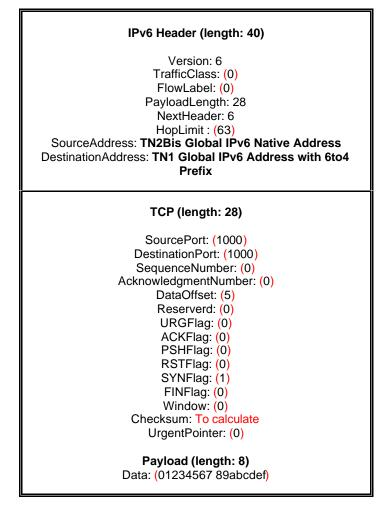
• IPv6/TCP Tunneled (length: 88 bytes)
