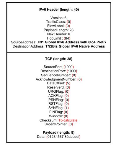
IPv6/TCP Tunneled (length: 88 bytes)
