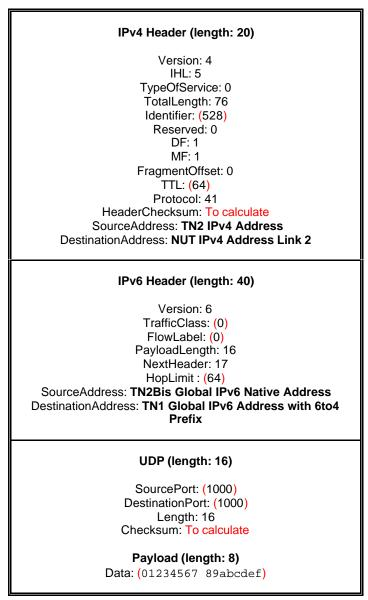
• Fragmented IPv4/IPv6/UDP Packet (2<sup>nd</sup> Fragment) (length: 44 bytes)
